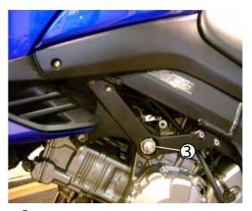
3 Now set a 17mm socket in place on the motor mount nut. You will turn this side while holding the right side.
