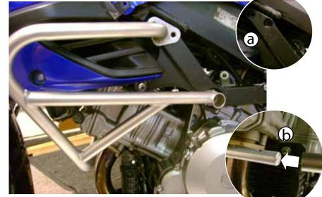
(a) Using a 6mm allen, remove the two top casting bolts.
