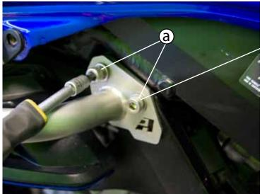
(a) Using a 6mm allen, insert the two M8 socket head cap screws (with M8 washers) into the top mount flange. Torque the M8s to 14 Nm (b) Replace the through-bolt nut and tighten until the locking nut engages the bolt.
