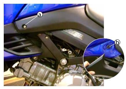
(a) Using a 4mm allen, remove the fastener on both sides of the bike.
