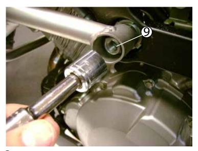
9 Torque the through-bolt nut down to 75 Nm.
