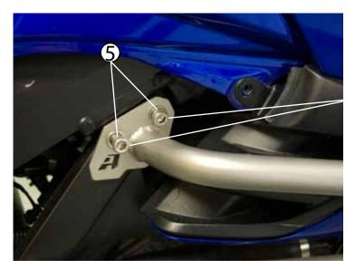
Put on the right side crash bar. Using a 6mm allen, insert the two M8 socket head cap screws (with M8 washers) into the top mount flange, and slide the through-bolt back in place. Torque the M8s to14 Nm.
