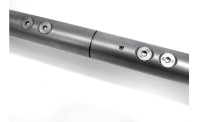
8 Using a 4mm allen, insert the flat head M6s into the four holes on the front underside of the assembly.
