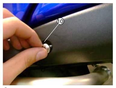
1 Put the plastic cover pieces back on both sides and reinsert the OEM fasteners. Do not over-tighten!
